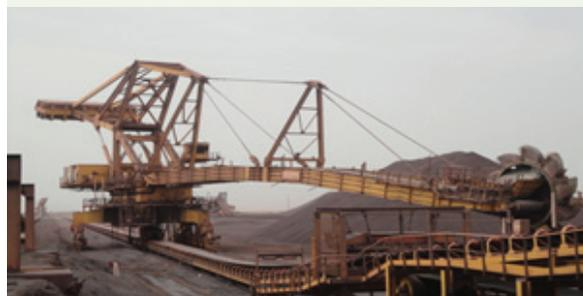
Bucket Wheel Reclaimer transporting ore to the ship
